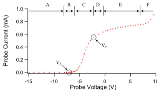
Figure 2: A representative Langmuir probe trace with different regions of interest indicated.
